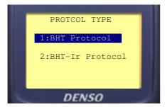
For BHT300 press 1 ENT to set Ymodem, then press C C C to return to the SYSTEM MENU
