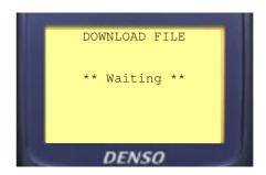
2) Transfer the new program (PD3 or PD4) file from the PC by running the Winartu3 shortcut (or selecting send on the Program Loader). The display will show the transfer progress and BEEP twice when completed. Now press **C C** to return to the SYSTEM MENU.
